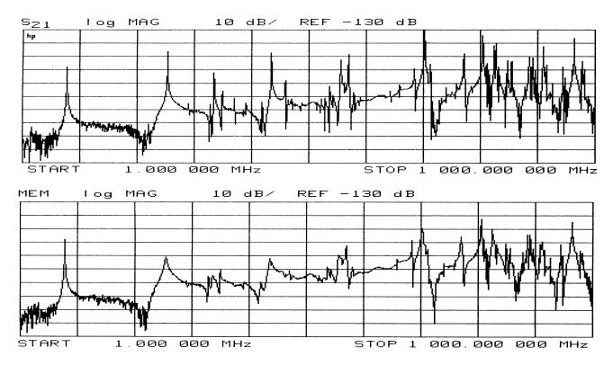
Figure 4. Frequency spectrum of the model cavity with (bottom trace) and without (top trace) HOM dampers
