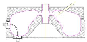
Figure 1. The CERN PS 80 MHz cavity shape (dashed line) and the TRIUMF wooden model with the coupling loop and the capacitive tuner.
