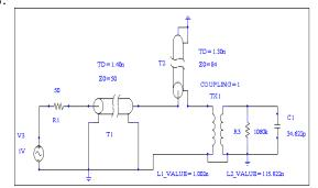
Figure 2. The equivalent circuit of the cavity-loop system
