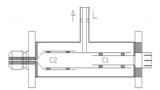
Figure 5. Transmission line design of filter
