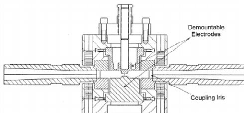
Fig. 4.  $TM_{020}$  RF breakdown test cavity assembly
