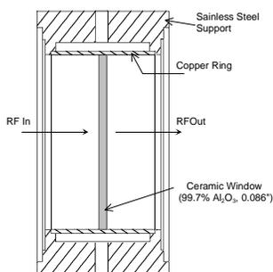
Fig. 5. Output ceramic window.
