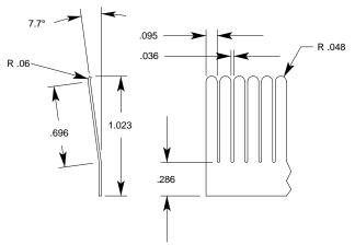
Figure 3. Spring finger Dimensions in Inches.
