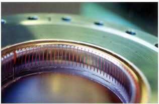
Figure 4. Spring Fingers as welded into Mounting
