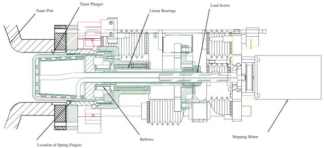
Figure 2. Tuner Cross-Section with Stepping Motor Drive.
