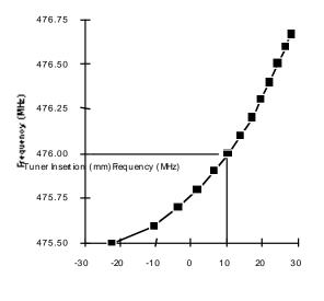
gure 6. Cavity frequency versus tuner insertion.
