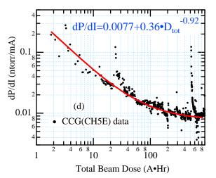
Figure 3. The beam induced dynamic pressure rise, (dP/dI), at various locations in the IR. (a) At Q1E chamber; (b) on the beamline next to the ISP chambers, and (c) for the soft-bend chambers. (d) shows dP/dI for a gauge within the hard-bend sector pumped only by distributed ion pumps, where the SR flux and gas load are the most intense.
