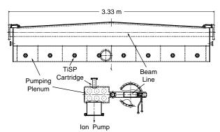
Figure 2. The Soft-Bend Chamber. Top view (above) and cross-section showing Ti pumping plenum.
