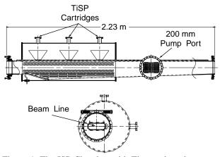
Figure 1. The ISP Chamber with Ti pumping plenum.
