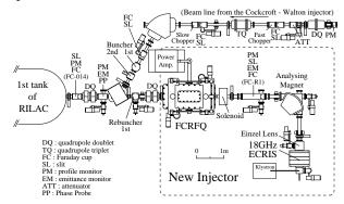
Figure: 1 Schematic drawing of the new injector for the RILAC
