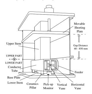
Figure: 2 Schematic drawing of the RFQ resonator. The inner volume of the resonator is about 1700 mm (length)  $\times$  700 mm (width)  $\times$  1150 mm (height).
