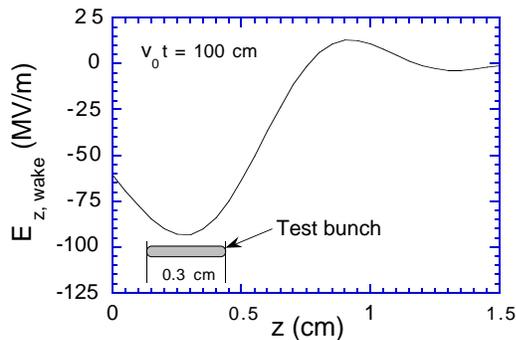
Fig. 3b. Location of the test bunch (bunch 11) in the accelerating wakefield near the entrance of the accelerator.
