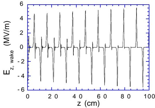
Fig. 2. Spontaneous wakefield from a -2 nC/mm, 30 MeV sheet bunch after it has traveled 100 cm left-to-right in the 2D waveguide depicted in Fig. 1.
