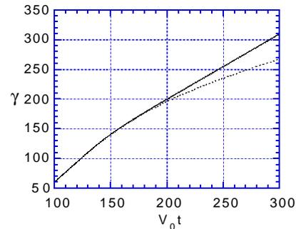
Fig. 5. Energy of test electrons versus  $v_0 t$  for two cases. Dotted line is the case shown in Fig. 4, but carried out for a 200 cm long structure, and the bunches are left in the system its entire length. Solid line is the case where drive bunches are removed after traveling 100 cm.
