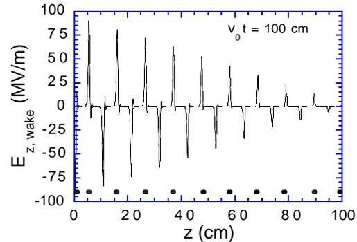
Fig. 3a. Cumulative wakefield set up by ten identical successive bunches, at the time the first bunch has moved 100 cm along the waveguide. The positions of the bunches are indicated by the heavy dots at the bottom.
