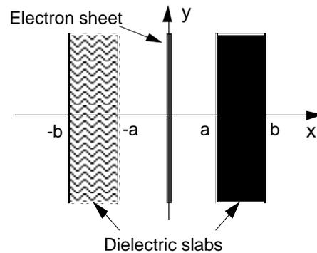
Fig. 1. Geometry for the 2D dielectric-lined waveguide.
