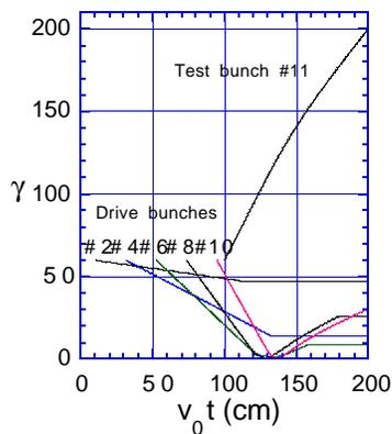
Fig. 4. History of the energy of selected drive bunches, and of the test bunch #11, up to the time the test bunch just emerges from the waveguide.
