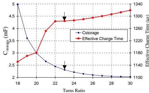
**Figure 5. Storage capacitor value and ECT as a function of transformer turns-ratio**
