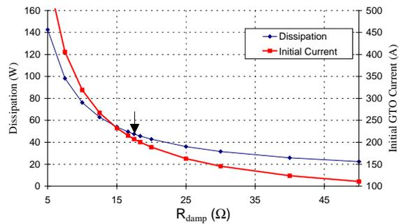
**Figure 4. Damping resistor dissipation and initial GTO current as a function of the resistor value**
