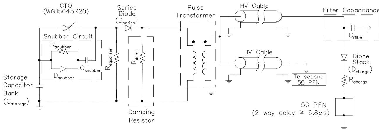
Figure 1. Schematic of Resonant Charging Supply
