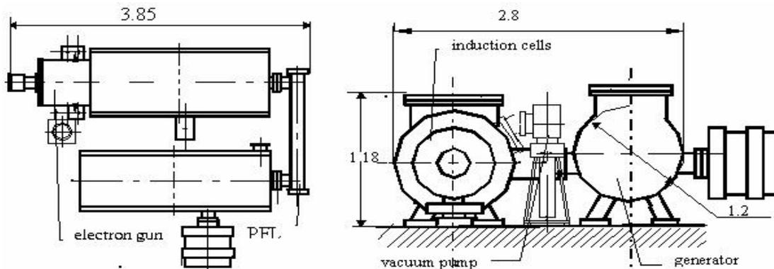
Figure: 1 The injector design.
