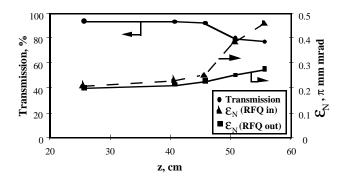
Fig. 5. PARMTEQM-calculated RFQ transmission (circles) and output  $\varepsilon_N$  (squares), and SCHAR-calculated RFQ input emittance (triangles) as a function of the distance between Solenoid #2 and the RFQ match point.
