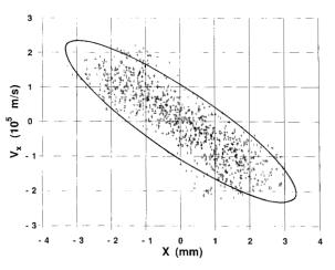
Fig. 3. SCHAR-calculated phase space (crosses) at the RFQ match point for the baseline LEBT design (Case No. 1). The curve is the RFQ acceptance ellipse for a 110-mA,  $0.20-\pi$  mm mrad beam.
