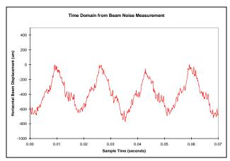
Figure 1: Horizontal beam position collected at 7.1 kHz.
