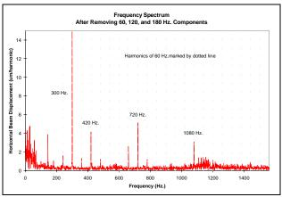
Figure 2: FFT following removal of 60, 120, and 180 Hz. contributions.
