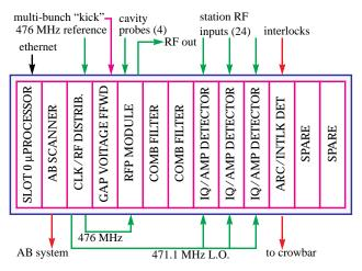
Fig. 1. PEP-II low-level RF system VXI crate topology
