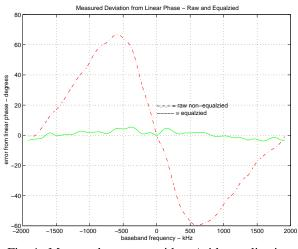
Fig. 4. Measured response without/with equalization.
