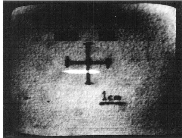
Figure 4: First beam spot observed at the Region 2 dump
