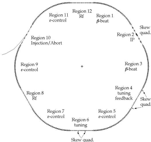
Figure 1: Layout of the High Energy Ring
