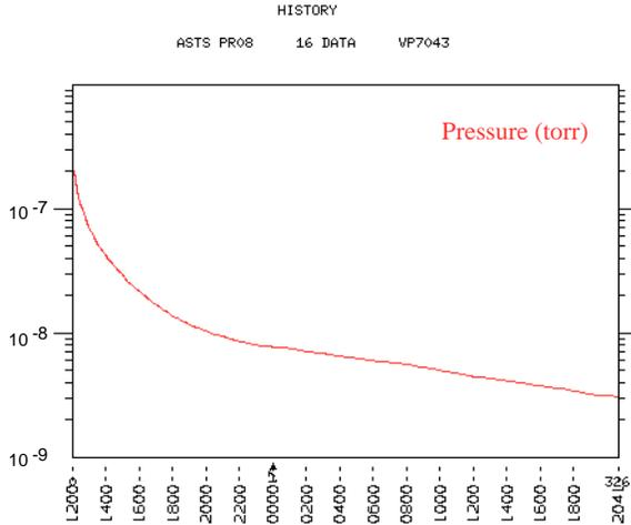
Figure 3: Initial pump down curve for Region 8.
