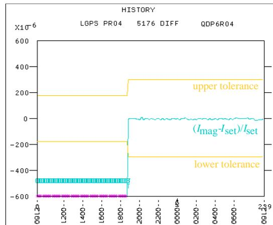
Figure 2: Power supply relative current variation vs time
