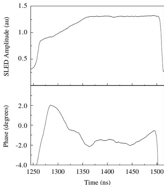
Fig. 3 Measured amplitude (top plot) and phase (bottom plot) of the SLED RF output in the linac for 13% beam loading compensation.
