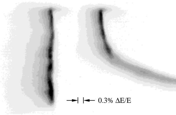
Fig. 5 Profile monitor images of the beam at the end of the spectrometer. The head of the bunch train is at the bottom and higher energy is toward the right (see text).
