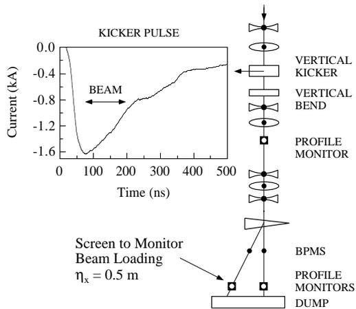
Fig. 4 Spectrometer layout and the kicker pulse shape.
