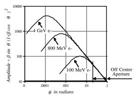
Figure 4: OTR Directivity versus spacial angle  $\theta$ .
