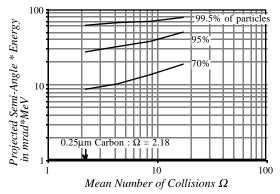
Figure 7: Plural beam scattering of highly relativistic electrons into thin materials. The number of collisions  $\Omega$  is equal to 0.78  $\rho t[(Z+1)Z^{1/3})/A$  where  $\rho$  is the density in  $g/cm^3$ , t the beam path length in the material in  $\mu$ m, Z the atomic number, and A the atomic weight.
