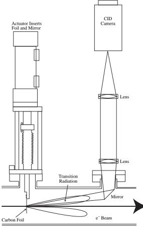
Figure 2: OTR profile monitor, top view.
