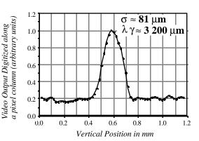
Figure 3: Vertical profile of a 3.245 GeV and 3  $\mu A$  continuous beam.
