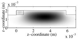
Figure 2: Gyroklystron cavity mode at 93.37GHz
