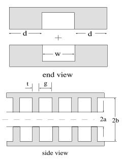
Fig. 1: Sketch of muffin-tin accelerating structure.
