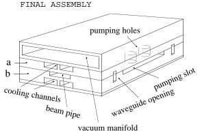
Fig. 5: Sketch of the 2nd generation design. Vacuum and cooling channels are included.
