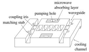
Fig. 6: Sketch of layer a — the top half of the structure.
