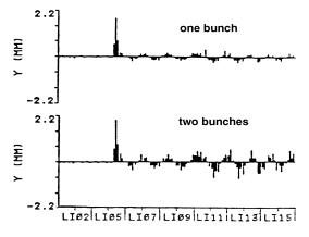
Figure 4: Wakefield kick of a 2 mm bump, top: for one bunch nearly closed, bottom: for two bunches a 250  $\mu$ m oscillation starts.
