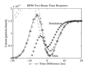
Figure 1: Measured (o) and calculated (\*) BPM response. Due to the slow rise time of pulses used in the test setup, the minimum is shifted to +2 ns, which can be also modeled (x). The dashed and dash-dotted lines in the top left, would be the curves, if the BPM were triggered externally and not self-triggered by the beam. The dashed curve is 1.5E10 (1-0.7 f(t)).
