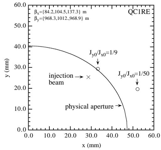
Figure 4: Physical and dynamic apertures at QC1RE. The origin is set at 44.55 mm from the center of QC1RE.
