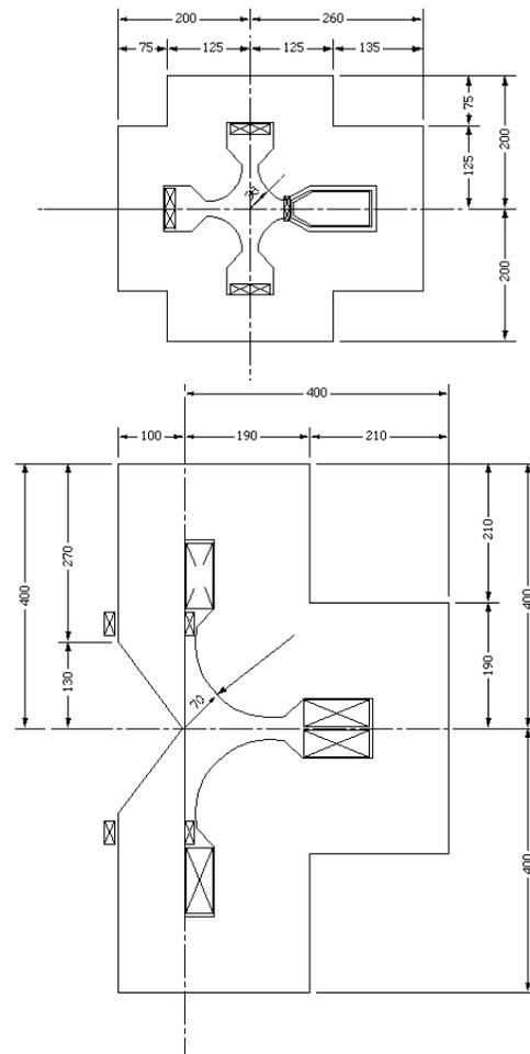
Figure 1: Schematic view of QC1LE (above) and QC1RE (below). A field free space is embedded in QC1LE. The other four quadrupoles have shapes like QC1LE.
