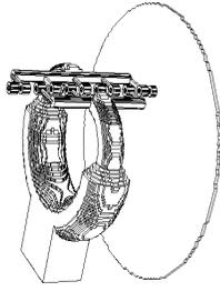
Figure 4: The SRIS short cavity. The outer cylindrical wall and front end one are not shown.
