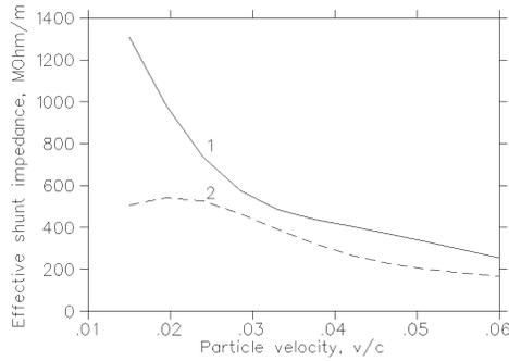
Figure 2:  $Z_e^r$  of the SRIS. 1 - for  $\beta \leq 0.03$ ,  $2a = 1.0cm$ ,  $\beta \leq 0.05$ ,  $2a = 1.4cm$ ,  $\beta \leq 0.06$ ,  $2a = 1.6cm$ ; 2 - for  $2a = 1.4cm$ ,  $2r_t = 3.0cm$ ,  $2r_c = 3.0cm$
