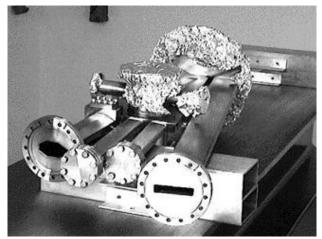
Figure 6: Dipole-1 outlet chamber
