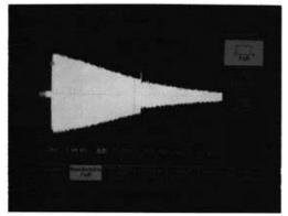
Figure 3: Strip line signal of the first stored 50 MeV electron beam in the synchrotron on April  $3^{rd}$  1997. Two injections 100 ms apart are visible
