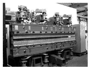
Figure 8: Undulater U49 ready for installation [6]
