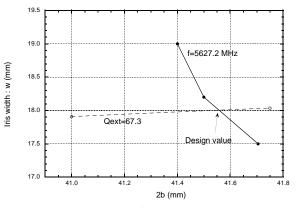
Figure 7: Determination of coupler dimensions
