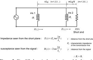
Figure 2: Simplified equivalent circuit model of two-iris coupler.
