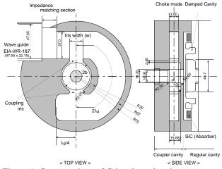
Figure 1: Cross sections of C-band accelerating structure.
