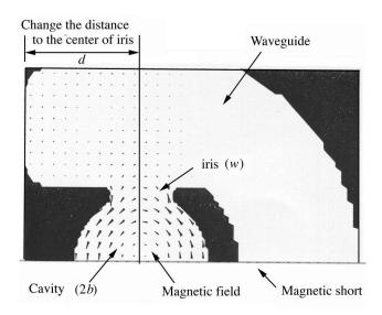
Figure 4: Cross section of the geometry used in Slater's tuning curve method in the plane normal to the beam axis. The whole geometry consists of the coupler cavity, waveguide, beam pipe, and half of 1st regular cavity.
