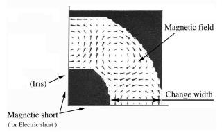
Figure 3: Geometry used in waveguide calculation by MAFIA. The arrows indicate the magnetic field under magnetic boundary condition.
