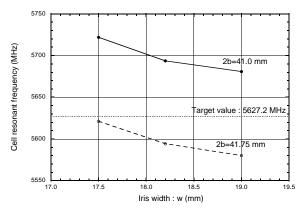
Figure 5: Resonance frequency of coupler cell.
