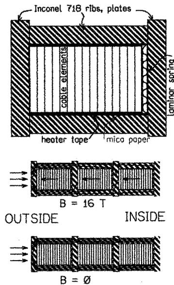
Figure 2. Detail of stress management in a coil block.
