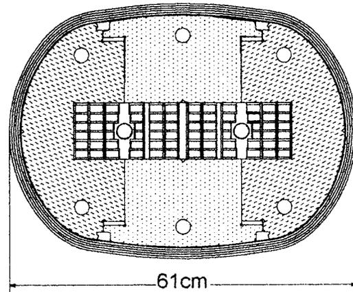
Figure 1. Block-coil dual dipole: 16 Tesla @ 4.2°K.
