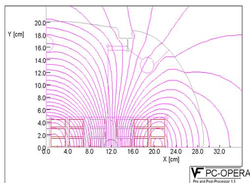
Figure 5. Calculated field distribution in 16 Tesla block-coil dual dipole.
