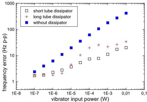
Fig. 2. Frequency error vs. vibrator input power.
