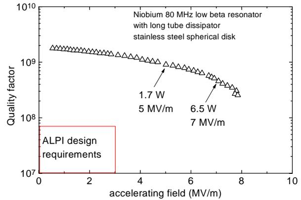
Fig. 3. Quality factor vs. accelerating field measured in the cavity equipped by a dissipator.
