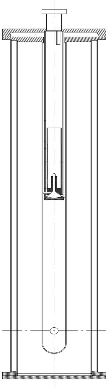
Fig. 1. Schematic of the mechanical damper inserted in a quarter wave resonator
