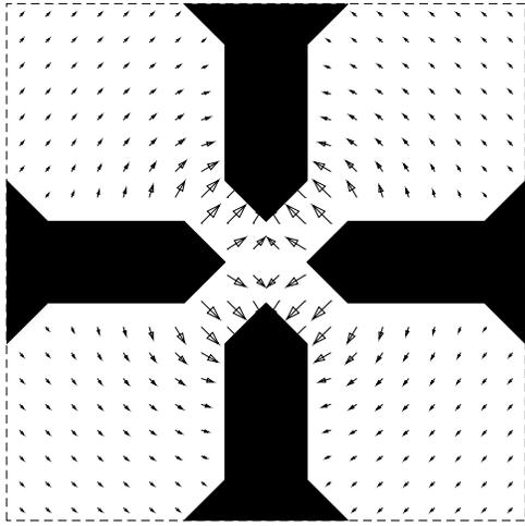
Figure 3: MAFIA plot of the electric field in a transverse section through the electrodes (detail).
