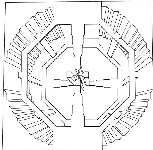
Figure 2: MAFIA plot of the 10 MHz RFQ (1 cell).
