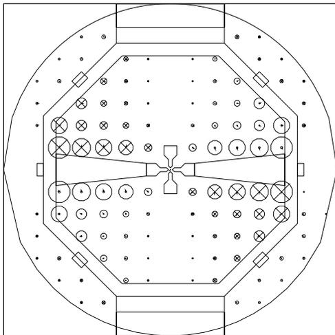
Figure 4: MAFIA plot of the magnetic field in a transverse section in the middle of a ring.
