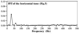
Fig. 6. Spectral analysis of the tune modulation
