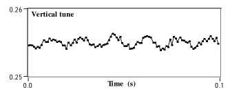
Fig.7 Modulation of vertical tune , no  $30\mathrm{Hz}$  power line interference
