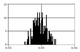
Fig.3 Distribution of horizontal tunes at 0 amplitude measured over 5 min. period at fixed phase relative to AC.
