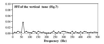
Fig. 8 Spectral analysis of the tune modulation
