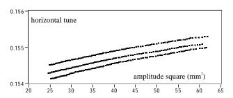
Fig.2 Horizontal tune vs. amplitude square for 3 consequent kicks.
