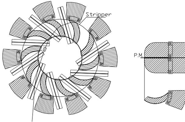
Figure 2: Layout of the 10 sectors RSC for 2 GeV H<sub>2</sub><sup>+</sup>
