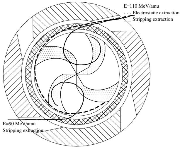
Figure 1: Layout of the 4 sectors CSC. The extraction trajectories for  $H_2^+$  by stripping together with the trajectory for fully stripped ions  $q/A=0.5$  extracted by electrostatic deflectors are shown
