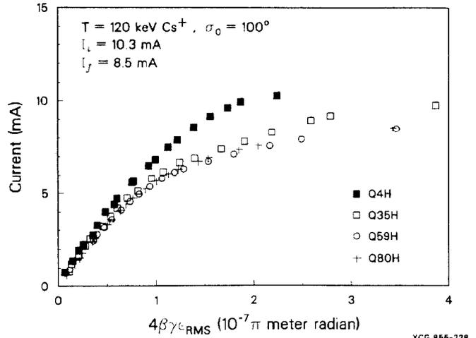
Fig. 3. Data obtained as for Fig. 2., but current drops as emittance initially rises. Collective effects drive particles from the core of the distribution and cause beam loss until apparently stable asymptotic distribution forms.
