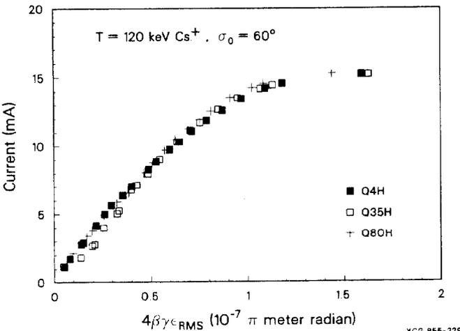
Fig. 2. From the measured  $(x, x')$  distribution of the beam at various lattice locations we calculate the RMS emittance and enclosed current of sub-distributions bounded by various intensity contours. Beam current is 15.2 mA, and emittance is well maintained through the lattice.
