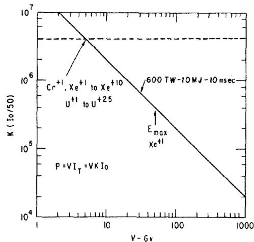
Fig. 1 Current multiplication factor vs. linac voltage for high confidence target case. Source current  $I_0$  is in mA.
