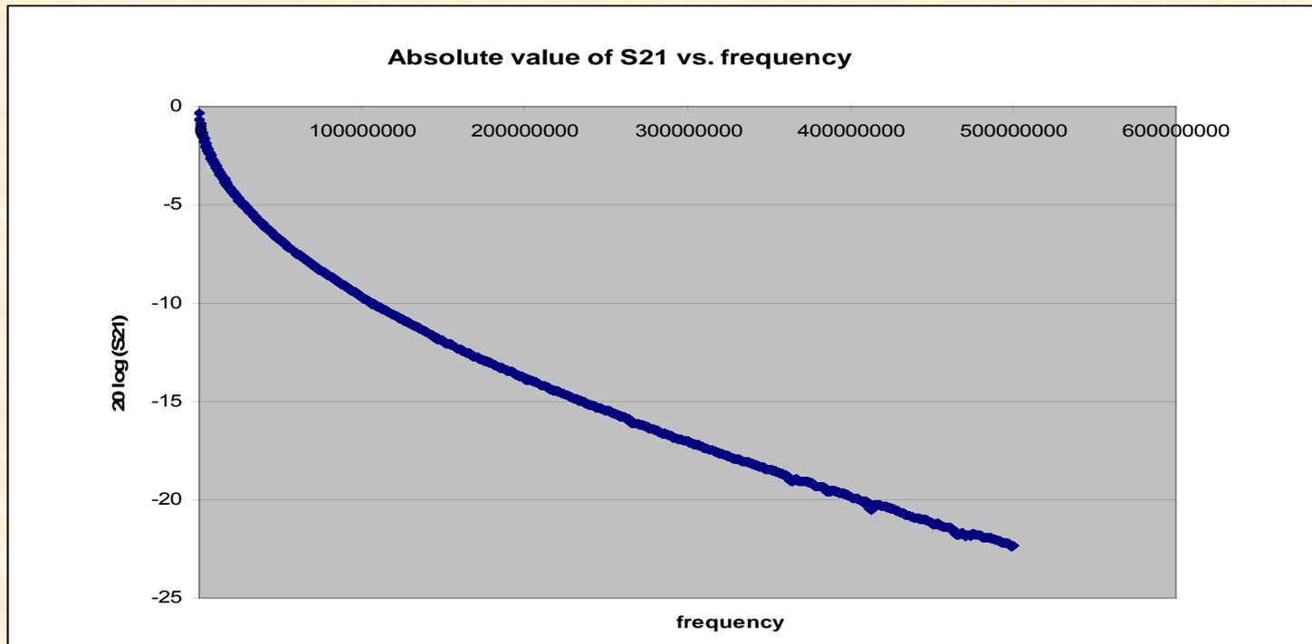
Characteristics of the measurement cable (in dB) vs. frequency
