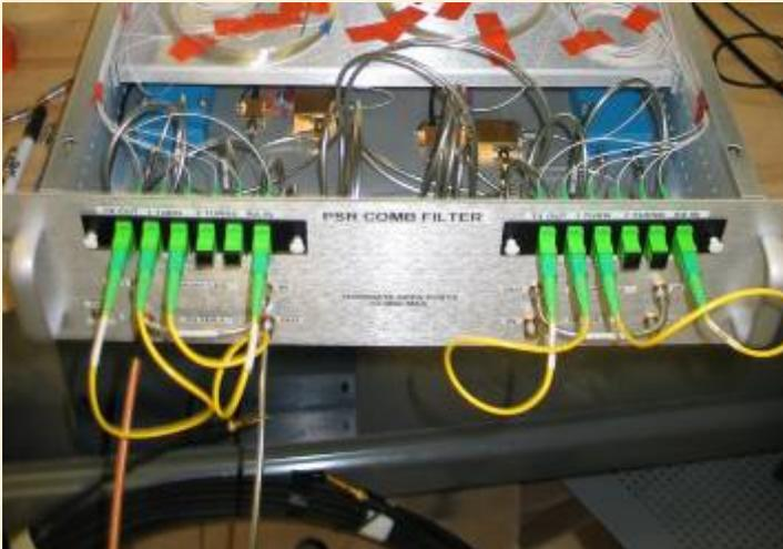
Long leg tuned to notch spacing accurate to better than 3 psec on average across the band.
