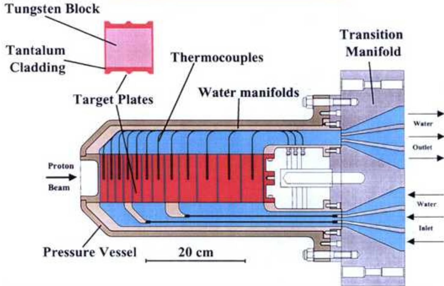
TS-1 tungsten target, tantalum coated, heavy water cooling
