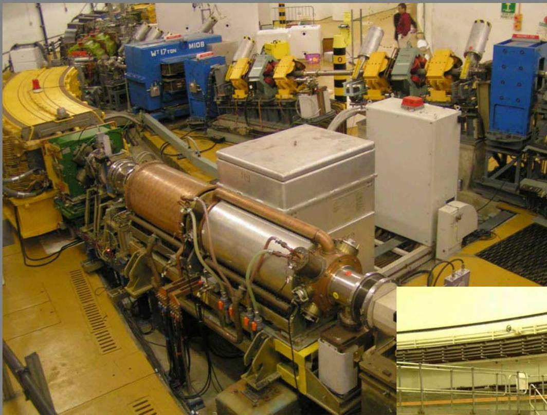
1RF accelerating cavity and high power RF driver
