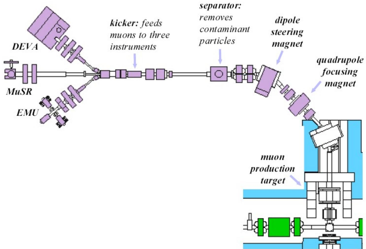
Muon production and transport — south side
