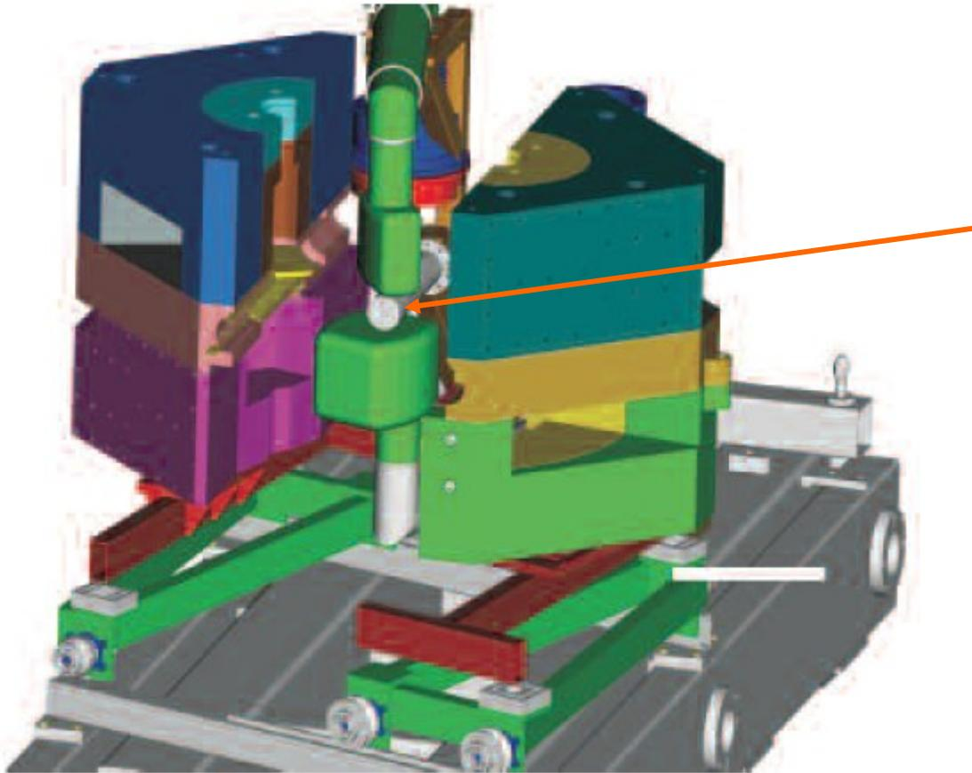
Solid tungsten cylinder, tantalum coated, surface cooled, 68 mm diameter — exploded view
