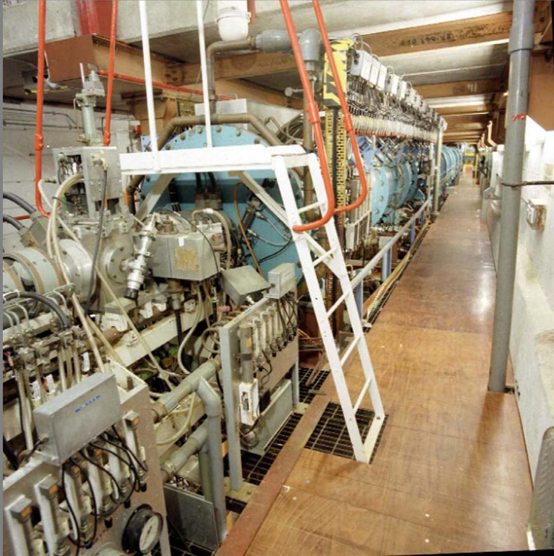
View down south side of 4-tank 70 MeV 202.5 MHz  $H^-$  linac
