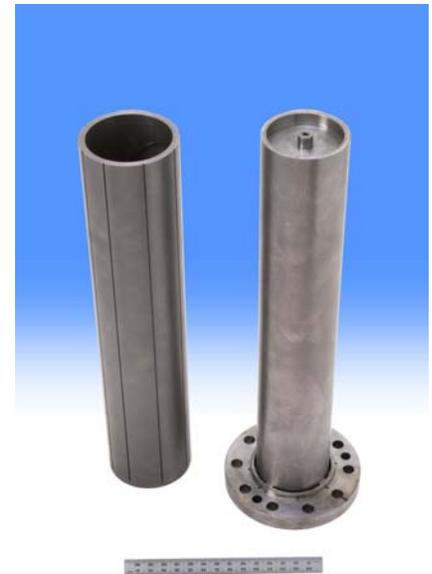
TS-2 tungsten target, tantalum coated, heavy water cooling
