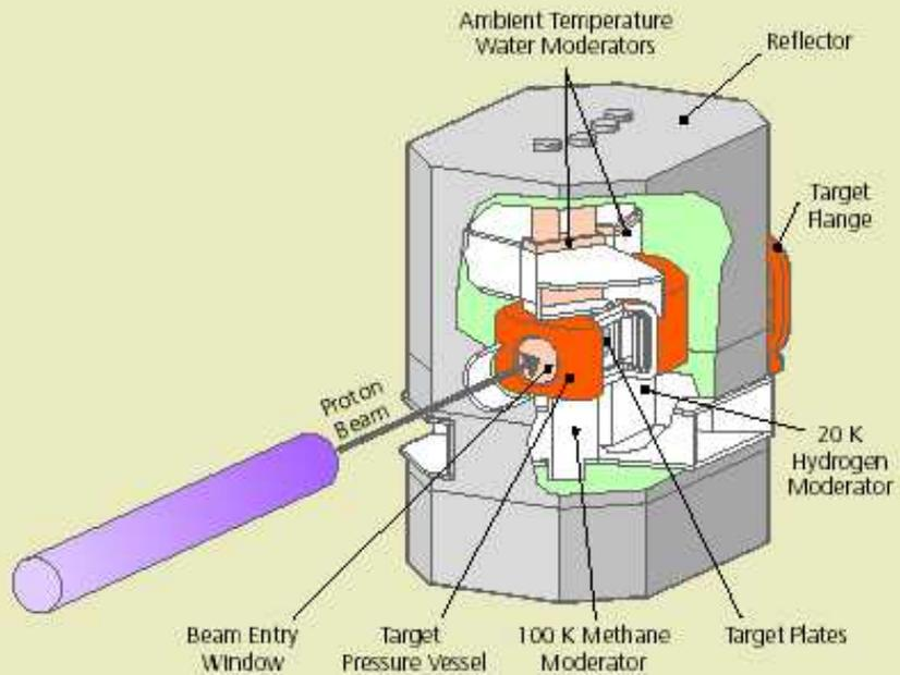
TS-1 target and moderator schematic
