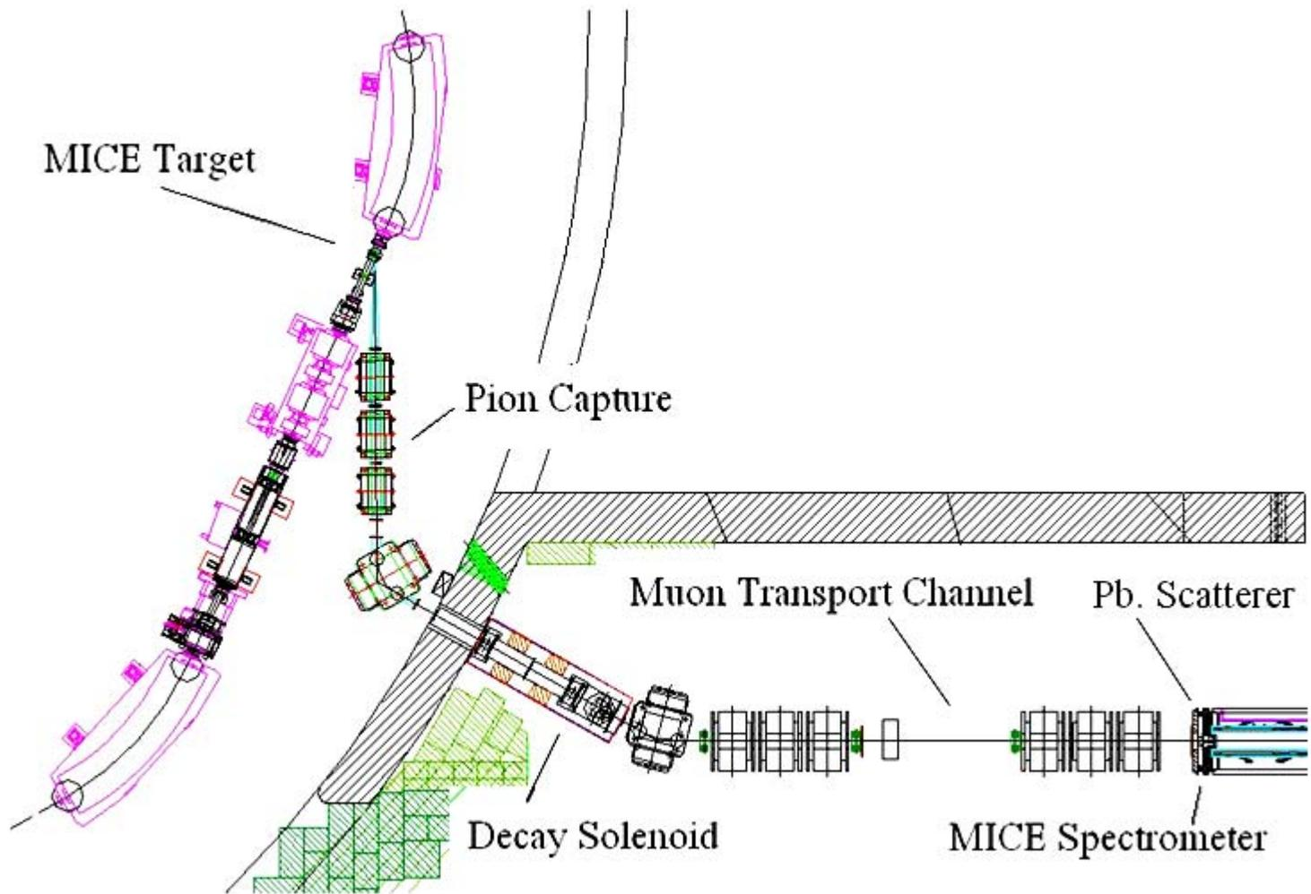
MICE beam line on ISIS synchrotron
