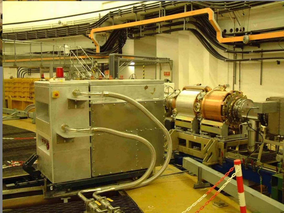
2RF accelerating cavity and high power RF driver
