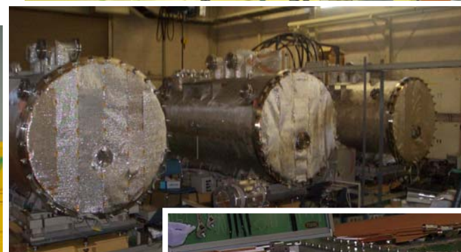
Kicker & Septum Magnets for fast extraction
