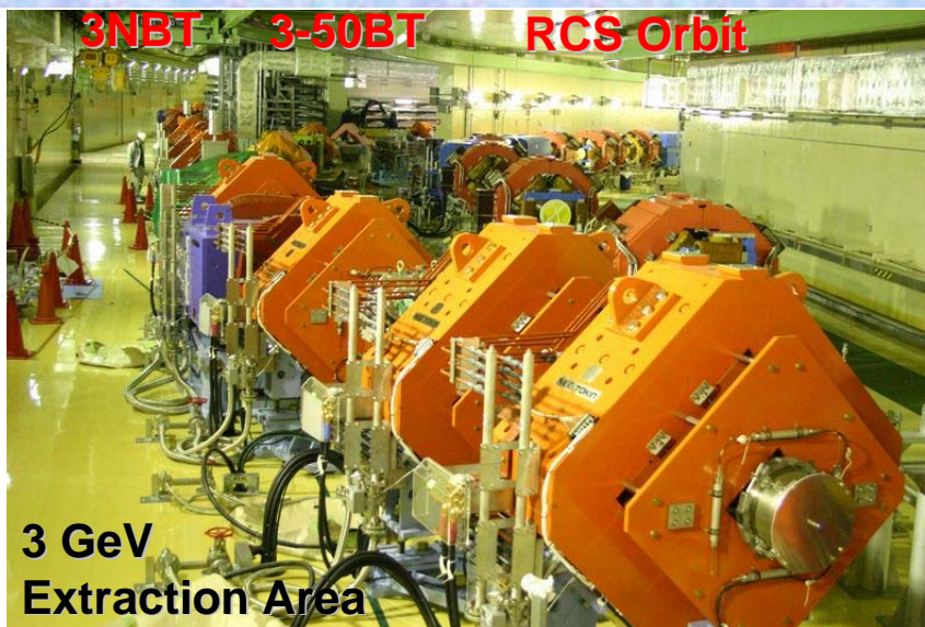
Kicker & Septum Magnets for fast extraction
