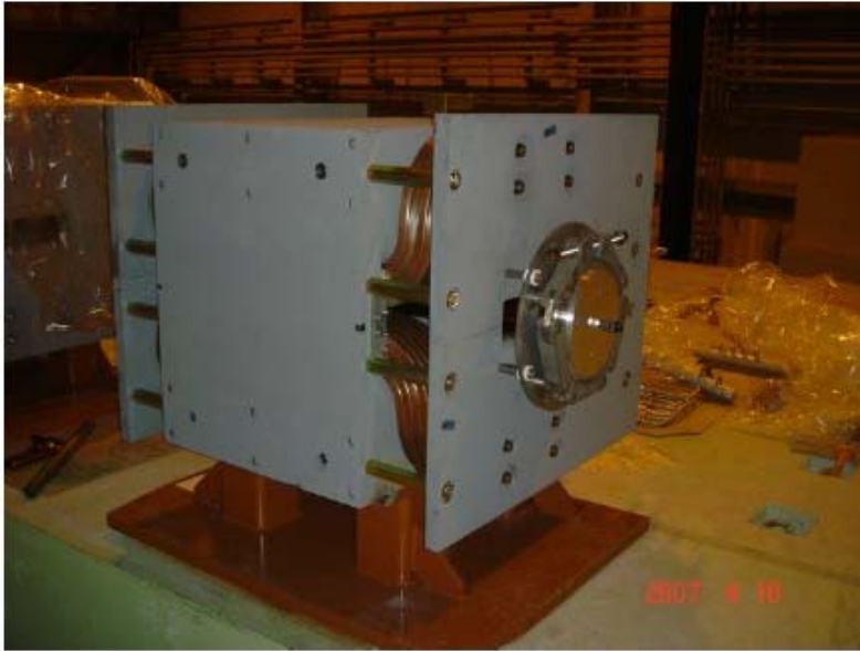
The first horizontal steering with a Ti-duct.
