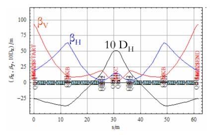
reduced drift in center, average 90°/cell -> negative dispersion at beginning/end  $\gamma_{tr} \sim 10$  i (for whole PS2)
