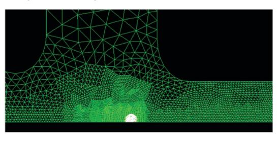
Adaptive refinement – Efficient simulations of long structures
