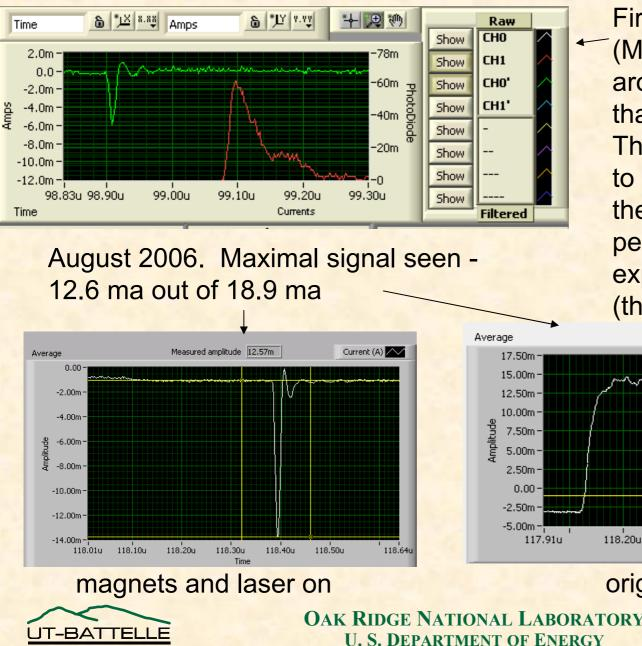
First observed signal (March2006) duration is around 10 ns –little longer than the laser one (7 ns) This was taken into account to estimate the actual stripping percentage. One hour experiment produced one (the only) set of data.
