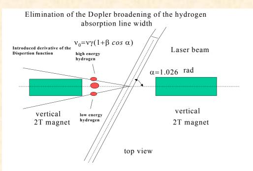
Dispersion function tailoring (dispersion derivative at IP) results in ion angle dependence on energy. 1 GeV SNS beam D'=2.58 for full elimination of Doppler spread of absorption line width due to energy spread
