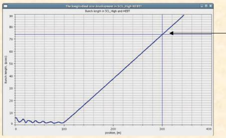
Linac bunch length too large (100 ps FWHM) Phases of last 6 cavities were optimized to squeeze the beam longitudinally. The length came out to be 10 ps (52 MeV energy drop) and 16 ps (4 MeV drop) (focusing is exchanged for energy)
