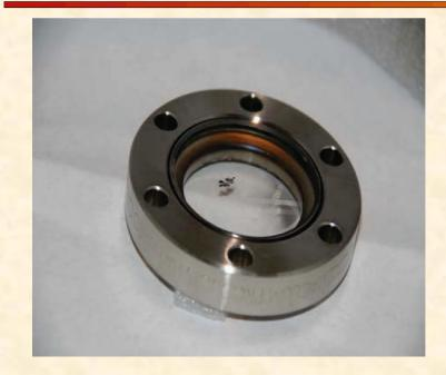
Powerful laser breaks the windows – in our experiment the laser density was reduced by factor 2 to prevent window damage. The maximal efficiency achieved when laser power increased to maximum and laser spot area increased two times
