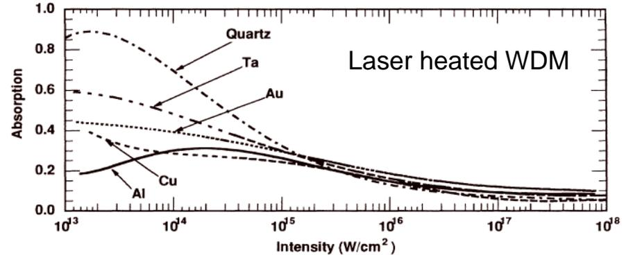
In quartz, electrons excited from 2s, 2p (ground state) to 3s leave holes in ground state to absorb photons in both cases. Measure decay rate of excited electrons by studying decay of absorption and emission rates.
