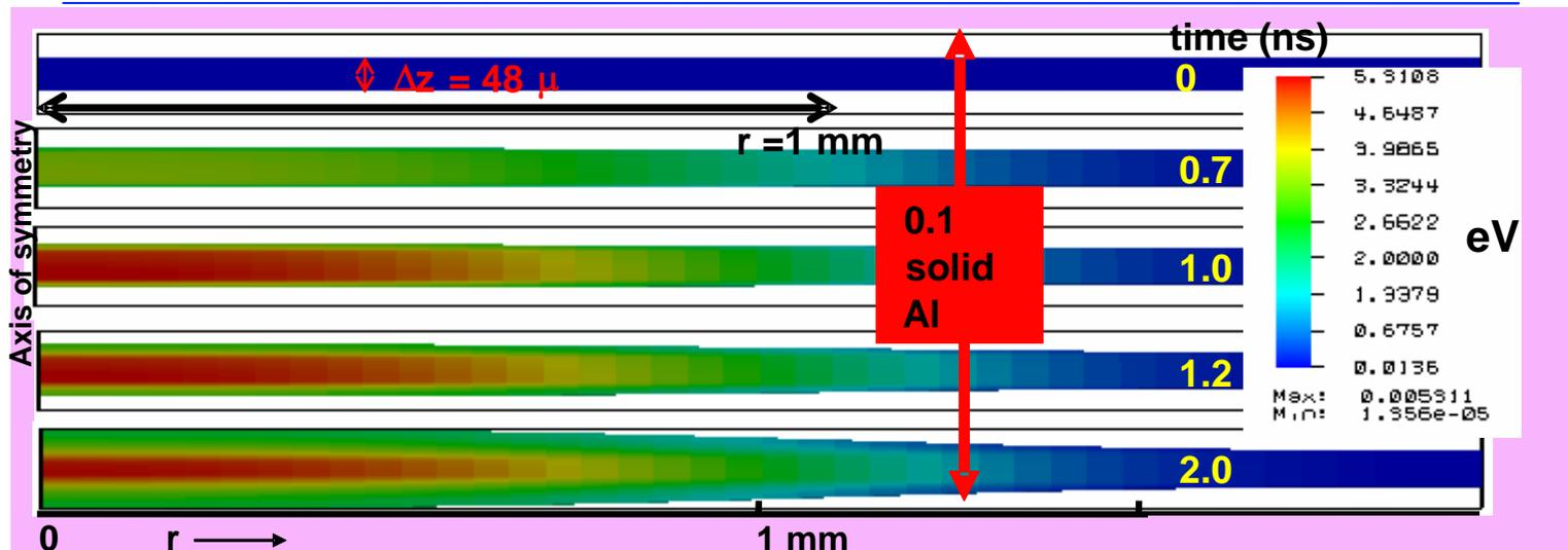
HYDRA model of beam heating in a porous target
