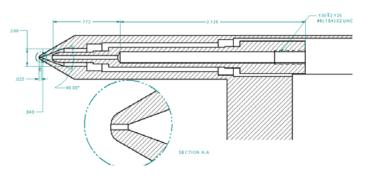
Carbon beam probe assembly
