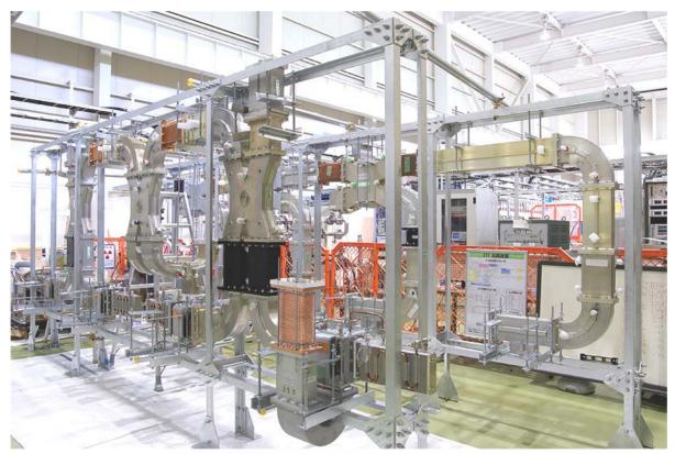
STF Phase 1: Two Cryomodules of Four Cavities Each
