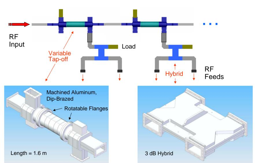
SLAC is building VTOs and custom hybrids and acquiring parts to assemble rf distribution systems for FNAL cryomodules
