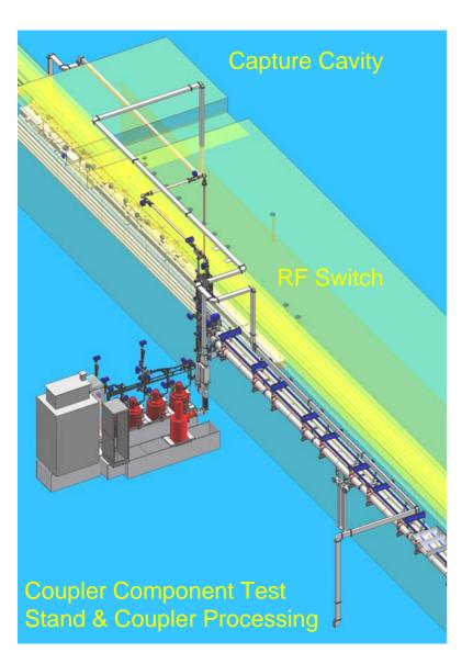
Produces 5 MW, 1.4 msec pulses at 5 Hz with a TH2104C klystron and a SNS-type modulator
