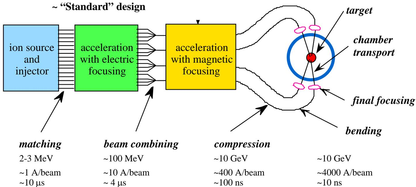
**Power amplification to the required  $10^{14}$ - $10^{15}$  W is achieved by beam combining, acceleration and longitudinal bunching.**
