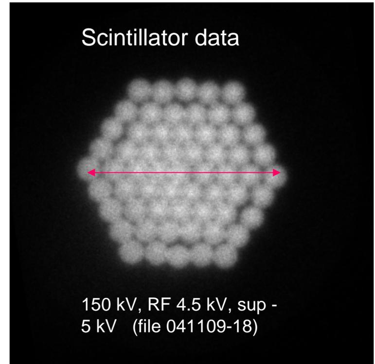
The overall cluster size and beamlet positions at  $z=15$  cm agree with simulation prediction but the individual beamlet profile is less sharp leading to slight overlapping at the central region.
