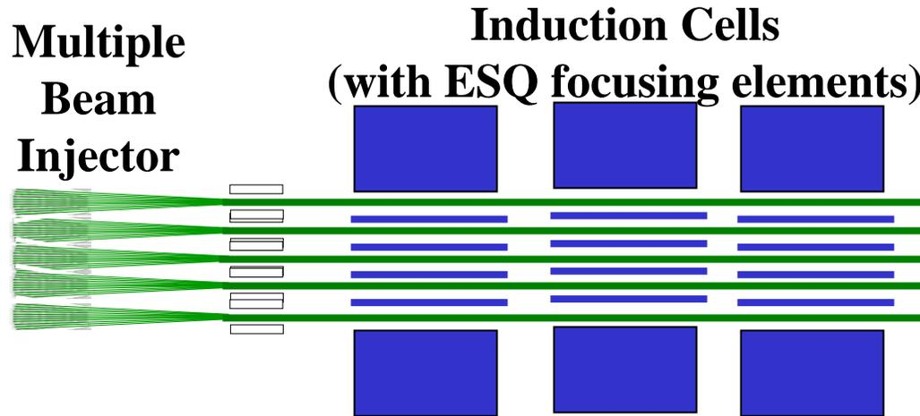
**At the injector, each beam has  $\sim 1$  A of current, and is  $\sim 20$   $\mu$ s in duration. Heavy ions are chosen to couple energy to the target without having large space charge fields in the final focus.**
