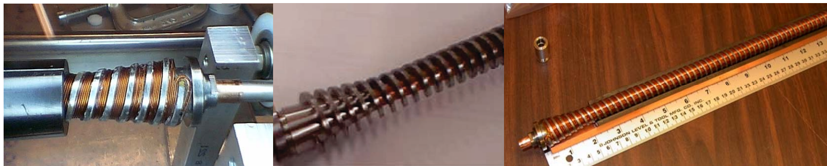
Fig.2:Details of design. 1–Iron yoke, 2–Copper collar, 3, 4–trimming Iron nuts. Inner diameter of Copper vacuum chamber is 8mm clear.
