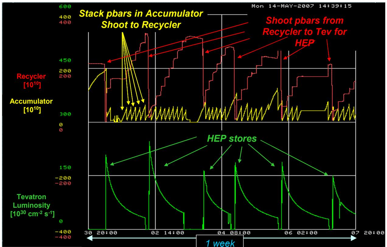
Figure 5: Antiproton intensities about the Fermilab complex.
