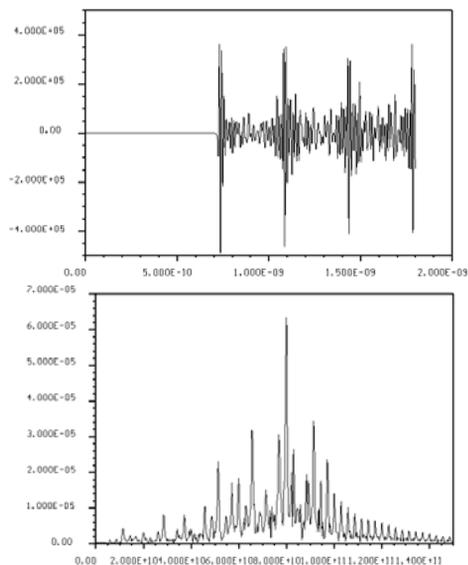
Figure 5: Examples: RF electric field at point 1 & frequency spectrum induced by 6 bunches
