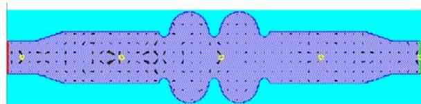
Figure 4: 6 Bunches are passing the cavity (the 1<sup>st</sup> one has passed through).
