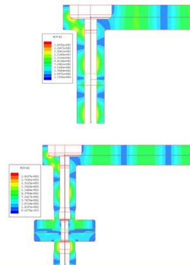
Figure 6: Straight Coaxial RF Coupler Section and Tapered Coaxial Coupler Section.
