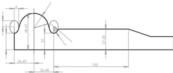
Figure 3: Cavity configuration after several series of optimization.
