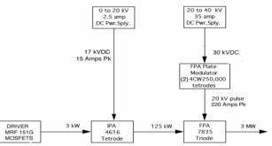
Figure 2: Schematic of the 201 MHz RF Amplifiers.
