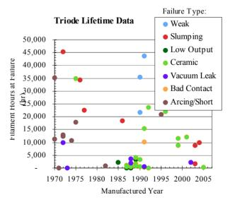
Figure 3: Summary of Triode Failures.
