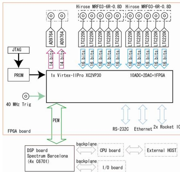
Figure 2: Schematic of the FPGA board.
