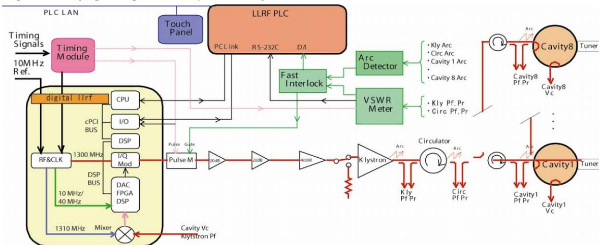
Figure 1: Schematic of the STF-LLRF system.
