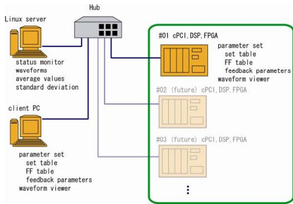
Figure 6: Schematic of LLRF data acquisition network.
