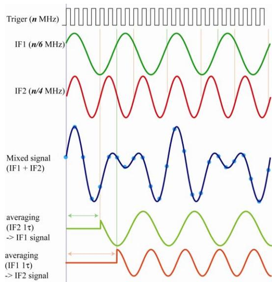
Figure 8: Concept of IF-mixture. By digital processing, two IF signals are restored.
