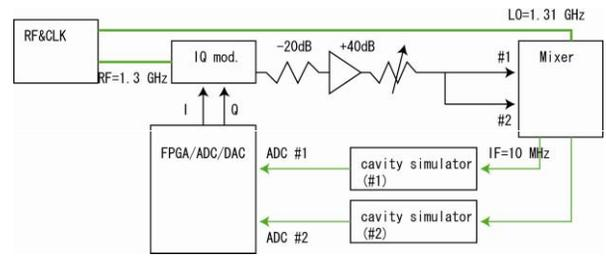
Figure 4: Performance test for the digital FB system.
