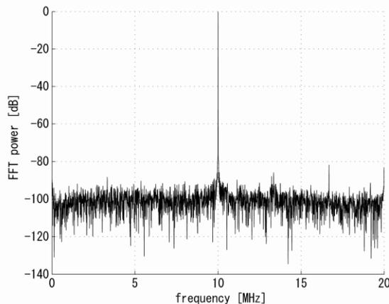
Figure 3: FFT spectrum obtained at 10 MHz input.
