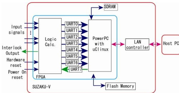
Figure 7: Interlock system using a Linux embedded FPGA.
