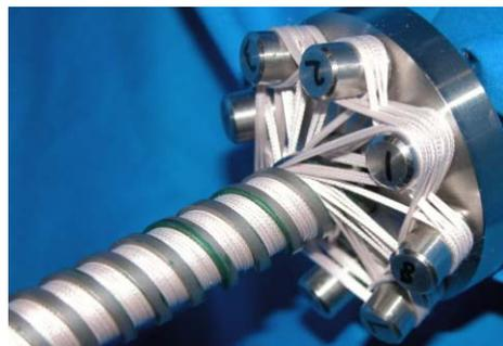
Figure 2: Undulator ends were designed for continuous winding of the double helix without any conductor joints. High-permeability steel poles were installed on the SS beam pipe before the coil winding.
