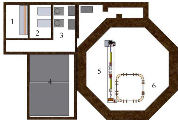
Figure 1: The schematic layout of ultra-fast source 1-control room 2-modulator 3-klystron 4-laser clean room 5-gun and linac 6-compact ring.
