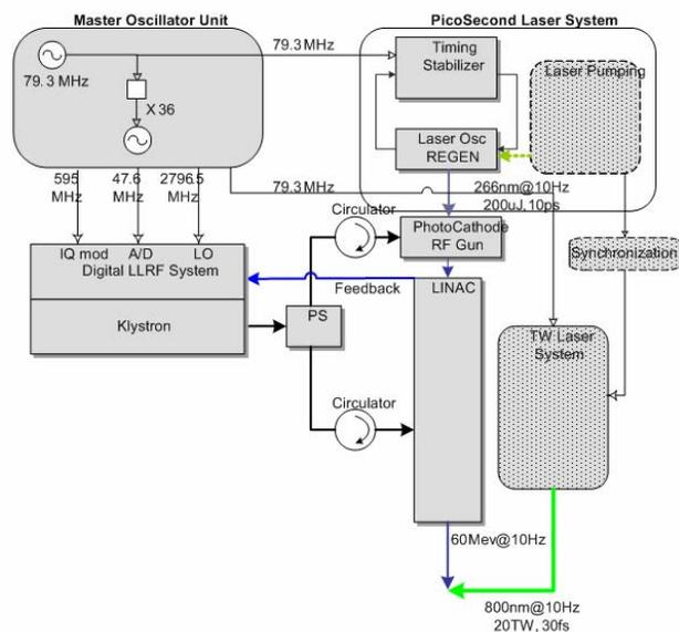
Figure 4: Conceptual design of synchronization
