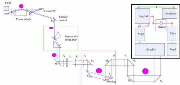
Figure 3: The schematic layout of driving laser system
