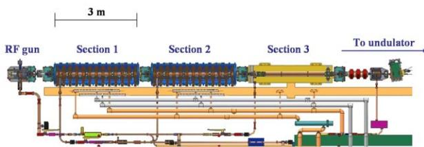
Figure 1: SPARC hall CAD top view.
