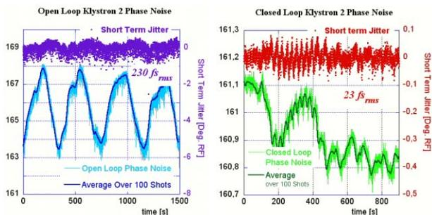
Figure 6: Open and closed loop RF station phase noise.
