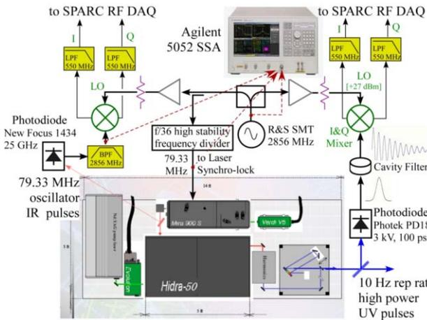
Figure 2: laser synchronization measurements.
