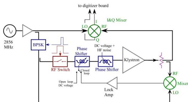
Figure 5: Intra-pulse phase lock schematics.
