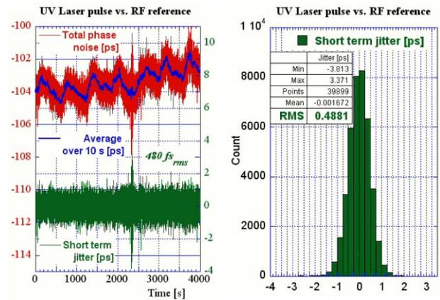
Figure 4: Phase jitter of the UV laser pulses.
