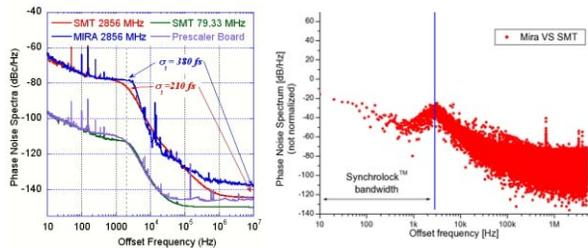
Figure 3: reference source and laser oscillator phase noise.
