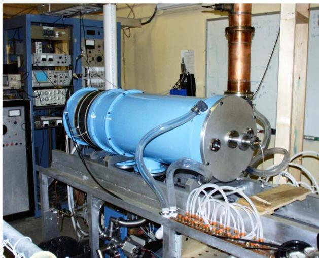
Figure 2. Photo of the injector in operating position with the 200-MHz, 750-keV RFQ.
