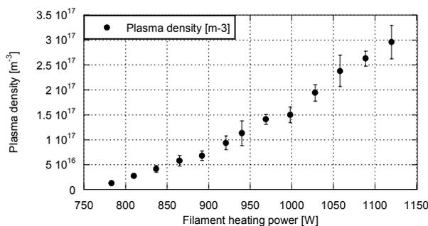
Figure 2 : Plasma density of the LANSCE filament-driven surface conversion  $H^-$  ion source (hydrogen plasma, no cesium)
