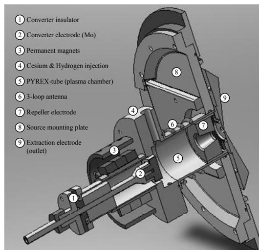
Figure 3 : Prototype of the helicon-driven surface conversion  $H^-$  ion source.
