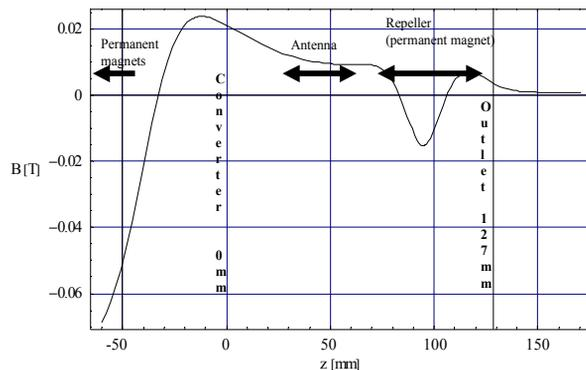
Figure 4 : The magnetic field on the axis of the source.
