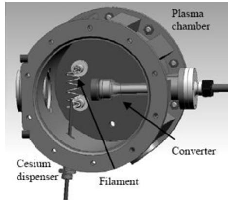
Figure 1 : Schematic of the LANSCE filament-driven surface conversion  $H^-$  ion source
