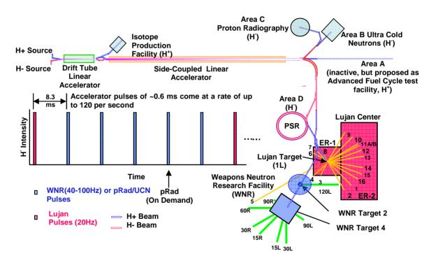
Figure 1: Schematic representation of the LANSCE User Facility at TA-53
