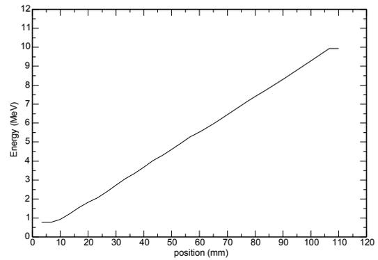
Figure 9: The energy gain of the proton bunch along the acceleration axis shows the energy increase during acceleration. The changes in slope in the figure (at 7mm and 107mm) are foils placed at the entrance and exit of the accelerator.
