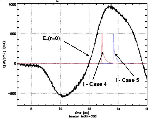
Figure 7:  $E_z$  (kV/cm) on axis and current (mA) 2.0 mm beyond the DWA entrance.
