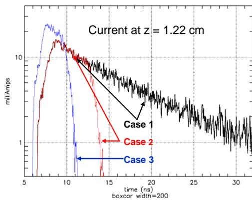
Figure 4: Total current just beyond the metal mesh.
