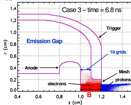
Figure 2: LSP model of the emission gap showing electrons cannot travel beyond the mesh.
